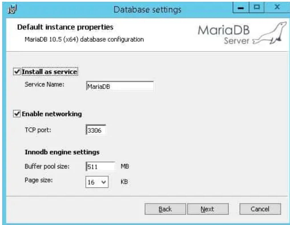
5. Please accept “Install as service” with MariaDB as the service name and ”Enable networking” on TCP port 3306 are selected and “InnoDB engine settings” with defaults settings.
