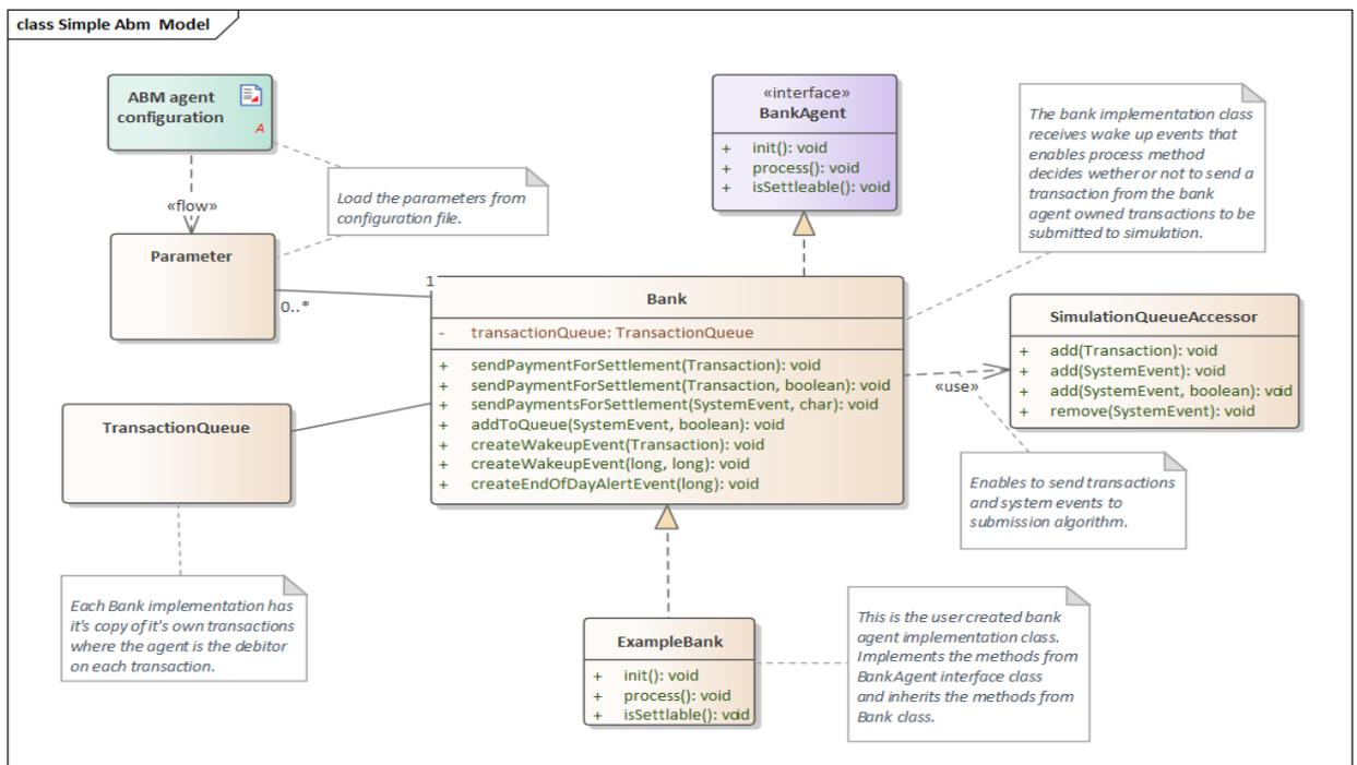
Please notice that all the other classes are existing simulator classes. At least in simple ABM implementations all the logic can be written to the new Bank child class. The methods listed for the Bank class are intended to be used when the derived bank agent class needs to communicate with the simulator's settlement process.
