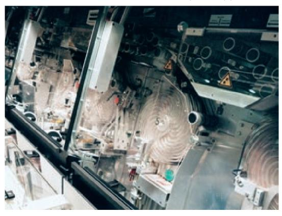
Fig. 25 Banknotes being sorted in central bank high-speed sorting machines. Their sensors check whether the notes are genuine and in good condition.
